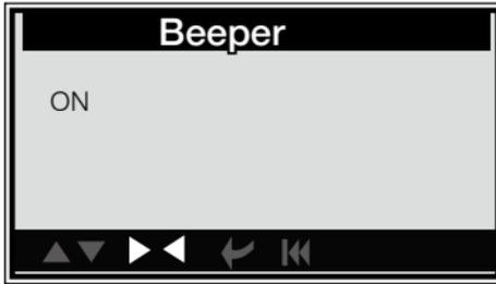
Press [UP] or [DOWN] to select ON/OFF and press [ENTER] to confirm.
