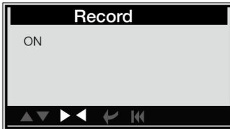
Press [UP] or [DOWN] to select ON/OFF and press [ENTER] to confirm. When this function is ON, and the icon record Datastream and record Freeze Frames.
